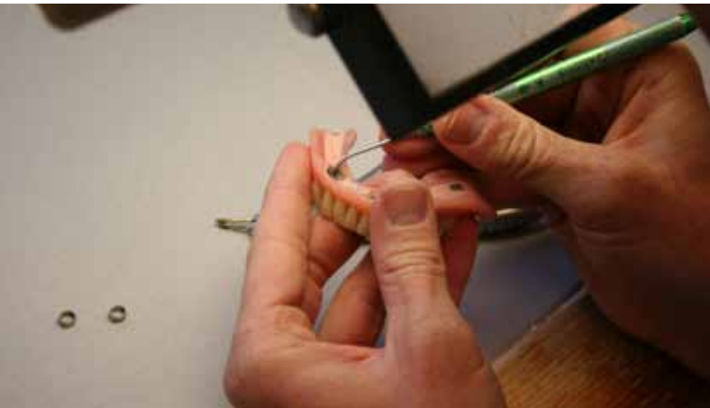
Fig. 11: Correcting the base after polymerisation.
